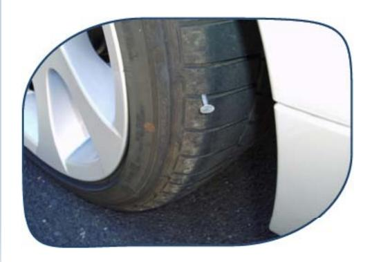
Detection = Nail in Tire (cavity)
