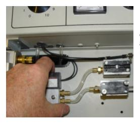
Fourth: Push the little, almost hidden, button at the top of the component immediately to the left of the pinch valve assemblies. This will cause the depressor (aka - pinch finger) to retract and make it much easier to install the new pinch tube.
