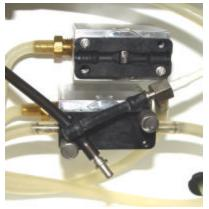
Third: Pull the pinch tube away from the bottom block and slip the old tube off the hose fittings.
