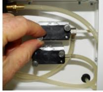
Second: Unscrew the finger tight screws to remove the top block
