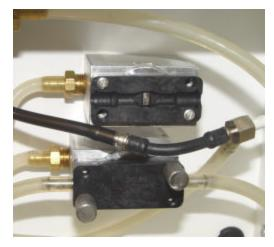
Fifth: Slip the new pinch tube onto the fitting and then seat the flanges of the fittings into the corresponding grooves in the bottom block.
