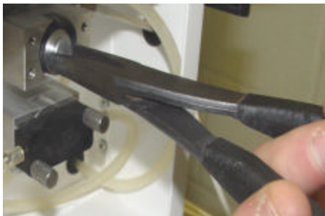
Extract Piston using needle nose pliers or simply turn on the machine and let air blow it out into the palm of your hand.
