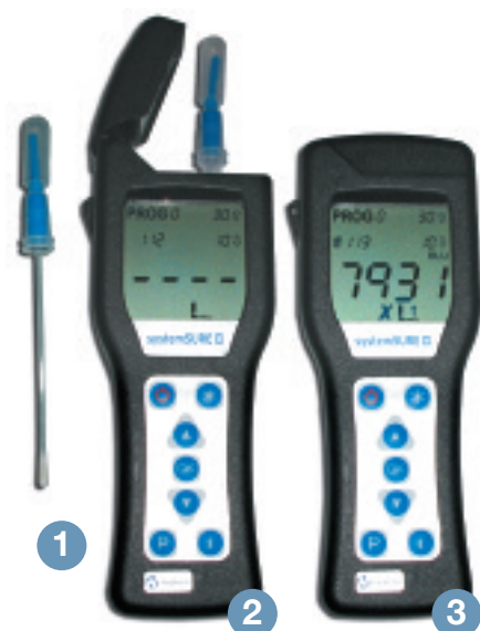
Fig. D The CariScreen test requires a swab (1) to be taken of the buccal surfaces of tooth Nos. 11 and 16. The swab then is placed into the tube, and the required chemicals are released by snapping the vial on the end of the swab. After agitating, the tube is placed into the light meter (2). The relative light units are displayed after 15 seconds (3). RLUs below 1500 are low caries risk; RLUs between 1500 and 2500 are moderate risk; and RLUs greater than 2500 are patients with a high caries risk.
